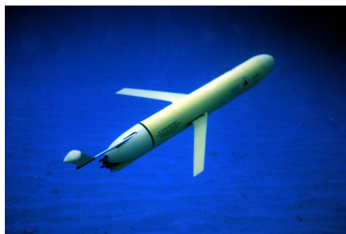
Figure 1: A SLOCUM underwater glider.
